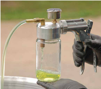
5. Pump sample into jar.
