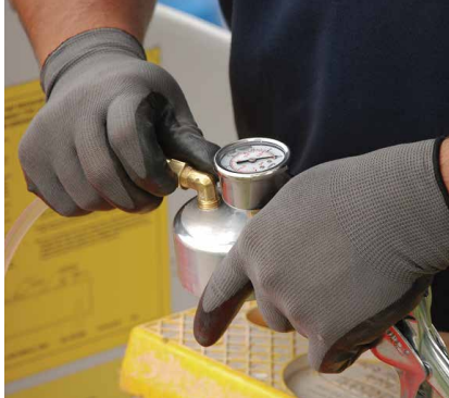
2. Attach the other end of the hose to the lid.
